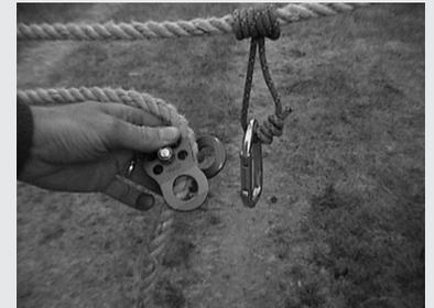
Using carabiners and pulleys can give you a mechanical advantage. Pulleys can exponentially reduce the amount of force needed to tighten the highline when used in multiples. Carabiners also can make attaching the highline components together fast and easy, and are handy in a pinch!
